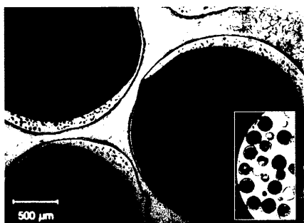
Fig 2: Fe-Cr hollow spheres in a 7075 Al alloy matrix. Inset: Bulk syntactic foam, spheres ~3 mm diameter.
